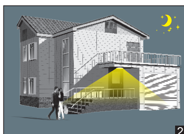
With insufficient ambient light, the sensor switches on the lamp when motion is detected.
